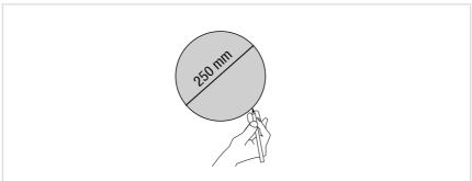
Cut a hole on the mounting location in the ceiling. Make sure the diameter is matching the cut-out measurement for the installing loudspeaker.
