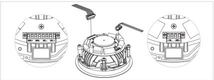
Connect the wiring by attaching the cables to the terminal block connectors and plugging them in to the CEL08S. Make sure the connectors are secured by tightening the set screws.
