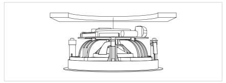
Make sure the mounting clamps are fully bended inwards, allowing the speaker to fit through the cut out. Insert the speaker into the cut out and tighten the mounting screws. A quarter turn is enough to flip out the mounting clamps, locking the speaker in place.
