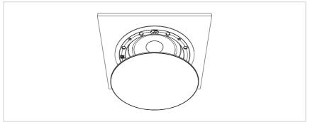
Attach the grill. Thanks to the magnets, it will snap in place.
