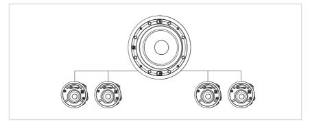
The CEL08S features an integrated stereo crossover, enabling you to connect your satellites. Two or four 8 ohm satellites can be used as well as eight 16 Ohm satellites.
